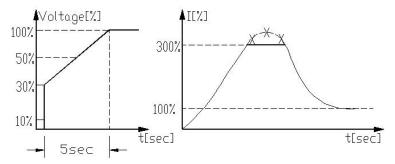
Voltage quickly increases to the INITIAL VOLTAGE value and then gradually ramps-up to nominal. Current simultaneously and smoothly increases to reach CURRENT LIMIT setting or less, before smoothly decreasing to the operating current. Motor speed will accelerate to full speed quickly and smoothly.
