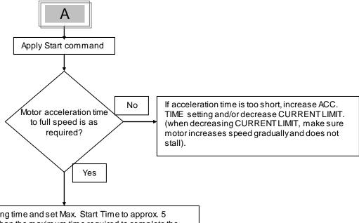
Check total starting time and set Max. Start Time to approx. 5 seconds longer than the maximum time required to complete the starting process.
