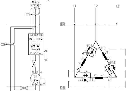
Reverse speed with RVS-DXM connected INSIDE DELTA.
