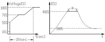
Voltage and current increase until current reaches CURRENT LIMIT. The voltage is held at this value until motor is close to nominal speed, then current will begin to decrease. The RVS-DXM continues to ramp-up the voltage until reaching nominal. Motor speed smoothly accelerates to full speed.
