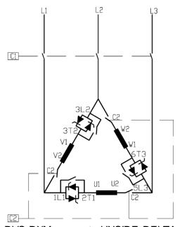
RVS-DXM connected INSIDE DELTA
