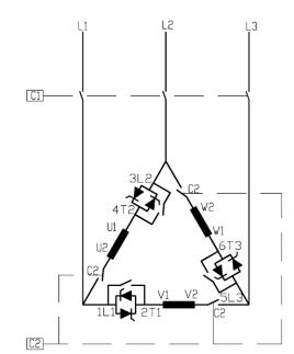
Speed reverse with RVS-DXM connected INSIDE DELTA
