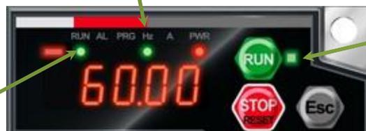
When RUN command source is keypad, the RUN-key is enabled and the RUN command indicator LED lights.
