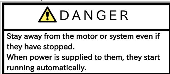
A rectangular label with a black border. The top section contains a yellow warning triangle with a black exclamation mark on the left, followed by the word "DANGER" in black capital letters. The bottom section contains the following text: "Stay away from the motor or system even if they have stopped. When power is supplied to them, they start running automatically."
