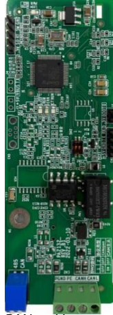
CAN multi-protocol communication card S1-CMS
