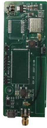
Bluetooth/WIFI communication card S1-BTx/WF
