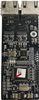
Ethernet/IP communication card S1-EIP / Modbus TCP communication card S1-EN
