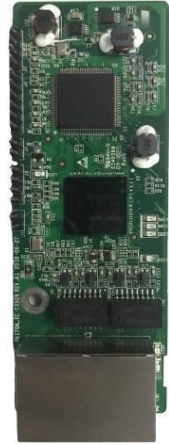
PROFINET communication card S1-PN
