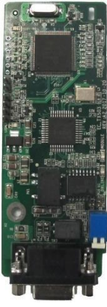
PROFIBUS-DP communication card S1-PB
