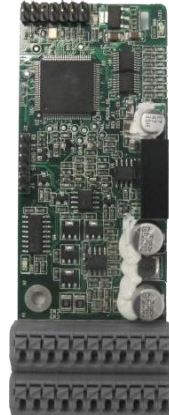
Resolver PG card EC-PG504-00
