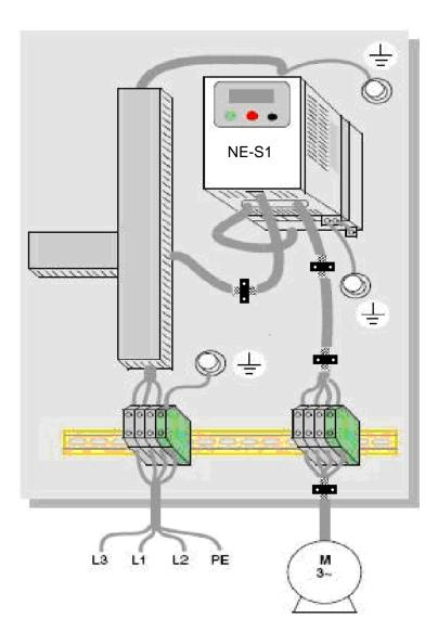
The following figure shows the required EMC compliant connection to the motor:
