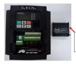
Removed optional board cover (Please carefully store an optional board cover. When the WJ-PN breaks down, it will be necessary for the temporary driving.)
