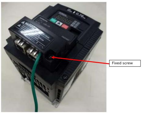
Please check the connection state of the WJ-PN and the WJ200 / WL200 inverter via the connector. When the connection state of the connector is bad, the Option error (inverter communication error, code: E6\*, please refer to Chapter 9) may occur after supplying power to the inverter. Or, because the inverter cannot recognize an option, normal communication may not be carried out.
