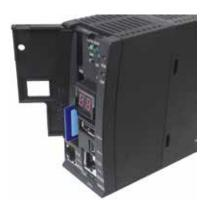
Large size data logging (SD Card) Removable SD Card provides a secure and simple way to maintain large data volumes for data logging up to 32 GB.
