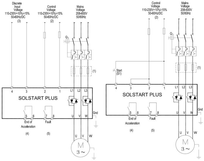
Control voltage and discrete input voltage from different sources.
