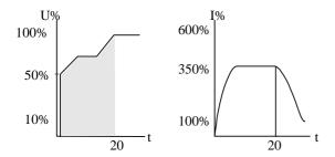
Upon Start the voltage and current increase until current reaches Current Limit value. The voltage remains at this value until motor reaches nominal speed, where current starts to decrease, voltage continues to ramp-up to nominal. At this time, the motor should have smoothly accelerated to full speed.
