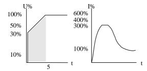
Upon start, the voltage quickly increases to the Initial Voltage value (30% Un) and then gradually ramps-up to nominal.
